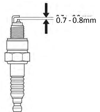
4. Measure the spark plug electrode gap with a wire type feeler gauge. Correct the gap, if necessary, by carefully bending the side electrode.
