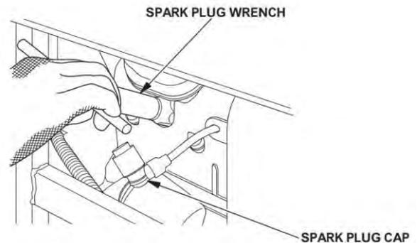
3. Inspect the spark plugs. Replace them if the electrodes are worn or if the insulator is cracked, chipped, or fouled.
