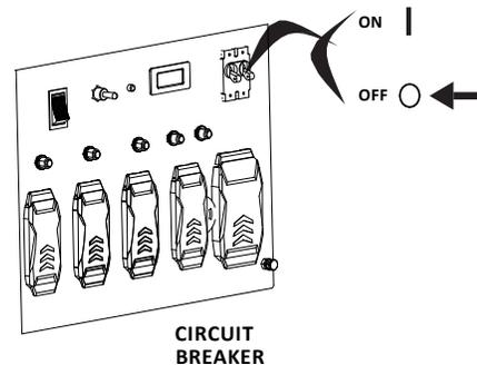
2. Turn the engine switch to the OFF position (when using gasoline).
