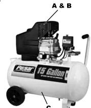
The pressure switch (located internally) shuts down the motor and relieves air pressure in the pump and transfer tube when the air pressure in the tank reaches the kick-out pressure. As compressed air is used and the pressure level in the tank drops to the kick-in pressure, the pressure switch restarts the motor automatically, without warning, and the pump resumes compressing air.
