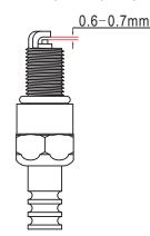
Standard Spark Plug: E6TC/E6RTC/BPR6HS
